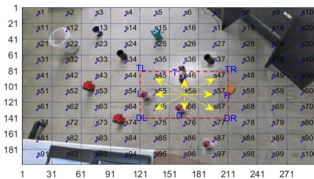
Figure 2. Path planning environment, including feasible, goal, and collision states. The arrows show the actions set 1. R: right, 2. TR: top-right, 3. T: top, 4. TL: top-left, 5. L: left, 6. DL: down-left, 7. D: down, 8. DR: down-right.
